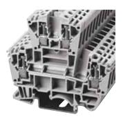
High-density connectivity using double-level terminal blocks. Marking system, side-insertion bridge and top screw-on bridge are standard. Use bridges to achieve any connection topology.
